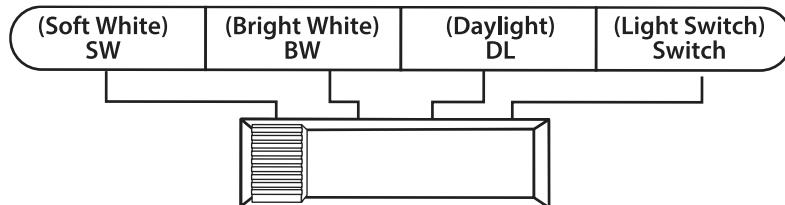
**NOTICE:** The toggle switch is located on the back of the fixture.
