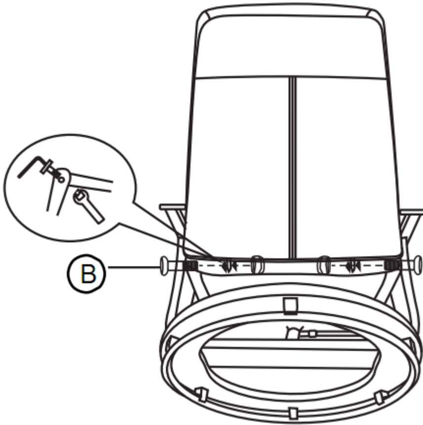
Secure Chair (1) to the Chair Base (2) with Connector Pins and Nuts (B).
