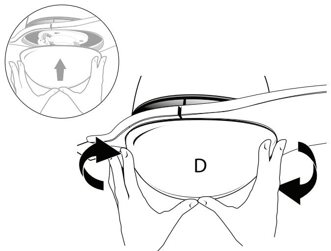
Locate the indentations on the neck of the glass (D) and align with the protrusions from the light kit. Lift the glass up allowing the protrusions to engage the indentations on the glass, and twist the glass clockwise to lock into place.
