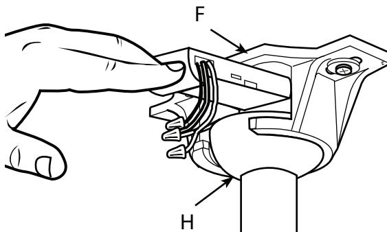
Align the keyholes on the canopy (E) with the protruding screw heads (S) from the mounting bracket (F). Lift the canopy up and rotate clockwise until the screwheads engage the keyslots fully.
