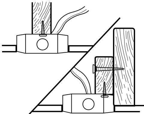
Install mounting bracket (F) to outlet box in ceiling using the screws and washers provided with the outlet box.
