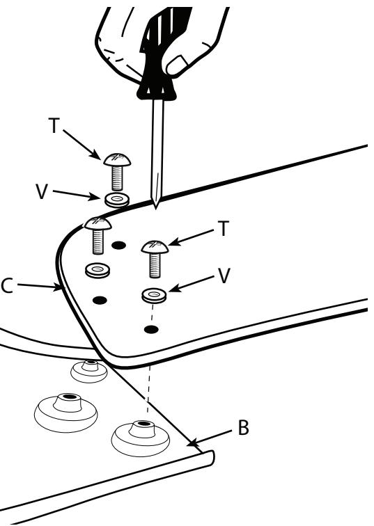
Attach blades (C) to the flywheel (B) using the blade bracket screws (T) and metal washers (V).
