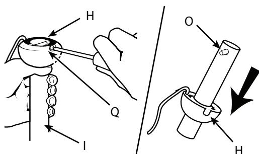
Re-install pin (O) into extended downrod, and slide downrod ball (H) up to the top of the downrod. Re-install set screw (Q) to secure ball to downrod. Note: Some extended downrods have a pre-drilled set-screw hole. If a pre-drilled hole is present in the extended downrod, tighten the set screw into the pre-drilled hole in the extended downrod. If no pre-drilled hole exists in the extended downrod, tighten the set screw against the downrod to secure the downrod ball. PROCEED TO STEP 6.
