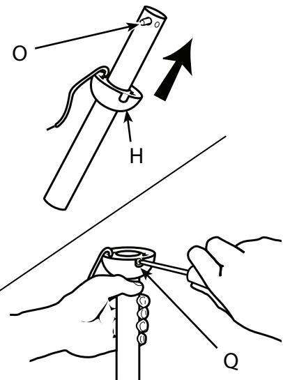
Carefully lift fan assembly onto mounting bracket (F). Rotate fan until notch on downrod ball (H) engages the ridge on the mounting bracket (F). This will allow for hands free wiring. See following step for wiring instructions.
