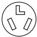
3-wire receptacle (10-30R)
