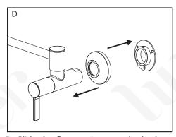
D. Slide the flange trim onto the body and attache the pot filler onto the pipe by turning the entire pot filler clockwise. (**IMPORTANT:** DO NOT overtighten the pot filler)
