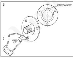
B. Place mounting base on the wall as shown in the figure with setscrew holes set at 12 and 3 o'clock positions. Mark the placement for the 3 screws with marker.
