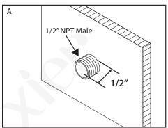
A. Shut off the main water supply before installation. The faucet requires an 1/2" NPT threaded male nipple extending 1/2" from the finished wall. For ease of future maintenance, it is recommended to install a shut off valve for the water supply line at an easily accessible location.
