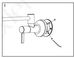
E. Tighten the 2 small setscrews with the hex wrench to secure the pot filler. Slide the flange to cover the mounting base after the pot filler is secured.
