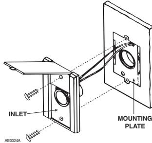
**NOTE:** If CF382S shorter radius elbow is used, it may be necessary to use the short mounting screw to avoid interference with elbow.
