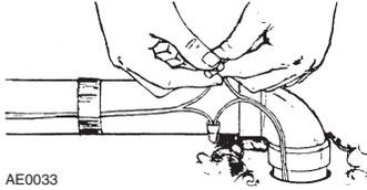
At the junction of every branch line and the trunk line, cut the trunk line wire and connect it to the branch line wire. Connect this wiring in groups of threes—one branch wire, one in-coming trunk line wire, and one out-going trunk line wire. Insulate all wire connections with electrical tape.
