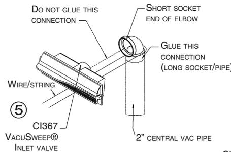
⑥ Remove the wire/string. With the door in an open position, secure the CI367 VacuSweep inlet valve to the cabinet base using no. 6 screws. Refer to figure ⑥. **Ensure that the spring on the electrical connector has 1/8" clearance to rough opening.** Continue with remainder of central vacuum connections.
