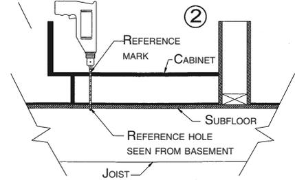
③ Cut a 2 1/2" diameter hole from the basement up into the base of the counter using the reference hole as a center. Refer to figure ③.
