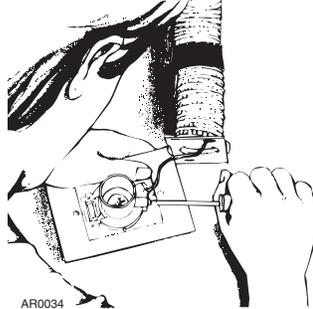
Insert the bottom screw into the inlet cover and through the other parts. Give the screw a few turns until it firmly engages in the mounting plate. Now, level and slightly lower the assembly. Make sure the wall is sandwiched between the inner and outer parts—you'll be able to feel if mounting plate is firmly centered on the inside of the wall.
