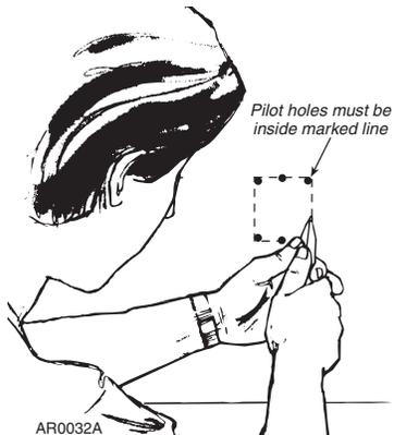
Next, use a keyhole saw or a sabersaw to make the cutout. Again, be extremely careful to cut along the inside of the marked line.
