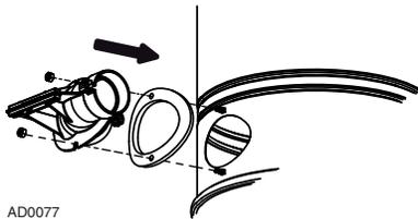
NOTE: Ensure the gasket is not folded in order to prevent lack of suction and noise.
