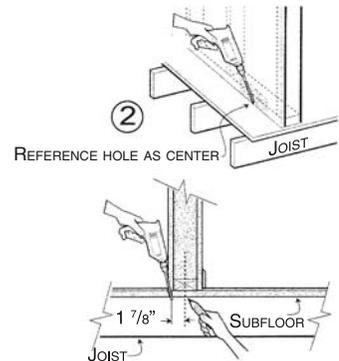
③ If installation is from below use a 2 1/2" diameter hole saw to remove wood floor and base plate, sufficient to locate CI367 VacuSweep inlet valve centered over the reference hole. Refer to figure ③.
