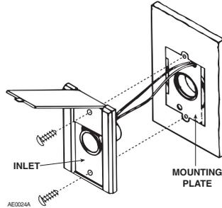
Hold the inlet in place and gradually tighten down each screw a little bit at a time. (If you completely tighten down one screw at a time, the mounting plate may pull away from the wall at the loose end and slip back into the cutout.)
