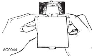
Holding the inlet assembly between your thumbs and fingers, angle the bottom of the mounting plate into the cutout. Push the assembly downward until you have clearance at the top of the cutout.
