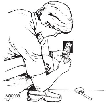
Now, remove the nail flange (used for new construction) from the inlet mounting plate. Use pliers to bend this flange along the scored lines until you can break it off.
