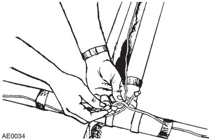
Complete all wiring connections up to the power unit's intake access hole. You will make this connection when you mount and connect the power unit. If, for some reason, you want to connect the wire as you go along, make the same two-wire and three-wire connections where required.
