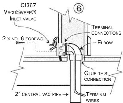
⑥ Remove the wire/string. With the door in an open position, secure the CI367 VacuSweep inlet valve to the wall using no. 6 screws. Refer to figure ⑥. **Ensure that the spring on the electrical connector has 1/8" clearance to rough opening.** Continue with remainder of central vacuum connections.
