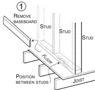
② Holding the drill at a 45° angle and as close to the wall as possible, between located studs, drill a small reference hole through the floor and subfloor. Locate this reference hole from beneath and measure over approximately 1 7/8" to center of base plate of wall. Ensure you have 1 1/2" clearance from any obstacles if connecting from below. Refer to figure ②.
