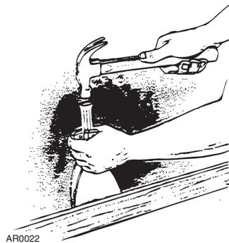
Directly below the inlet location, drill a 1/16" reference hole through the floor into the basement. (If you're drilling through carpet, use an awl to slightly open the weave. This will keep the carpet from wrapping itself around the drill bit.) Insert a piece of scrap wire or a clothes hanger into the reference hole so you can easily find the hole in the basement.
