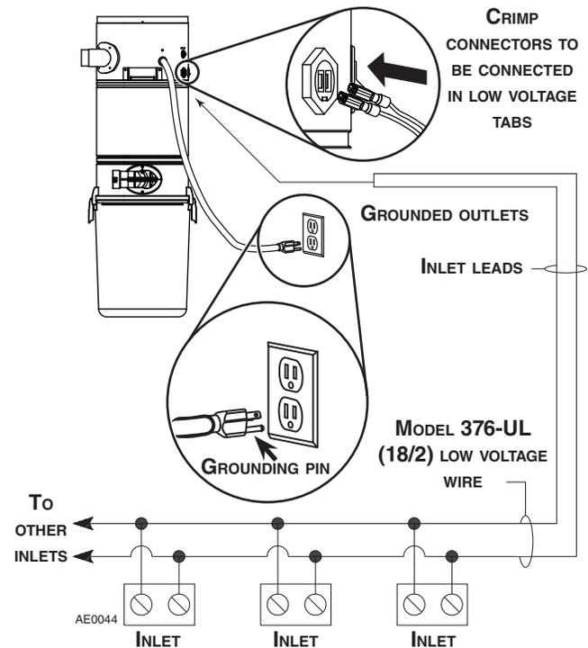
NOTE: Inlet leads to be connected to power unit low voltage tabs using crimp connectors (included in parts bag) and low voltage harness.
