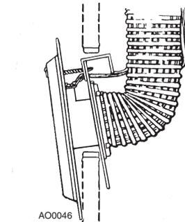
Push the top of the mounting plate into the cutout and lift the assembly upward until the top screw seats in the predrilled hole. At this point, the wall should be sandwiched between the mounting plate and the frame plate.
