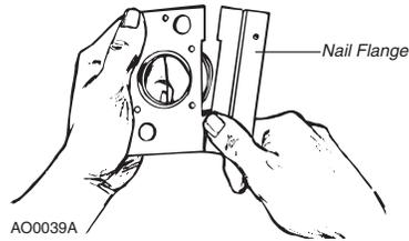
Apply cement to both the inside of the flexible tubing and to the outside of the mounting plate's tube ring. Insert the mounting plate's tube ring in the flexible tubing and twisting the pieces as you join them to spread the cement, and align the mounting plate in a vertical position.
