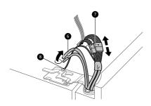
**3** Rotate the hinge lever **9** counterclockwise. Lift the top hinge free of the hinge lever latch **①**.
