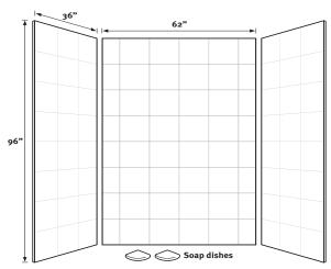
Designed to fit base areas 36" deep or smaller x 62" wide x 96" high or smaller (914 mm x 1575 mm x 2438 mm)
