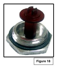
Screw the regulator cap back into the regulator and re-attach the regulator to the nipple and flare union. (See Figures 12 and 19)
