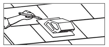
4. Trace outline of roof flange onto shingles.
