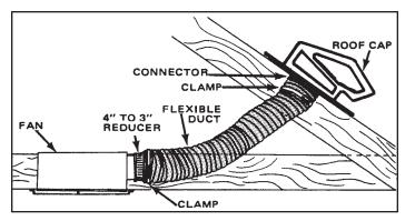
1. Cut a 5" diameter hole through roof boards and shingles.
