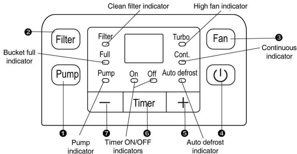
Control Buttons: whenever a button is pressed, the unit will make a beep sound to indicate that it is changing modes.
