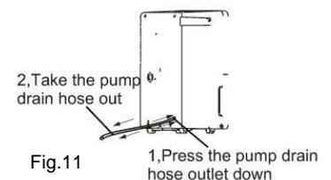
Note: Do not use Pump operation when outdoor temperature is 32°F or below. Water may become iced and block the drainage, leading to unit failure.
