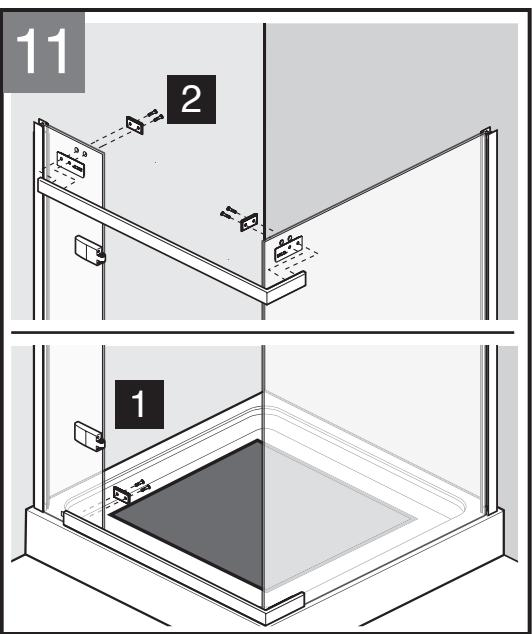
Attach bottom support bar to the small glass panel using the plastic spacer on the outside of the glass. Use the metal bracket on the inside of the glass.
