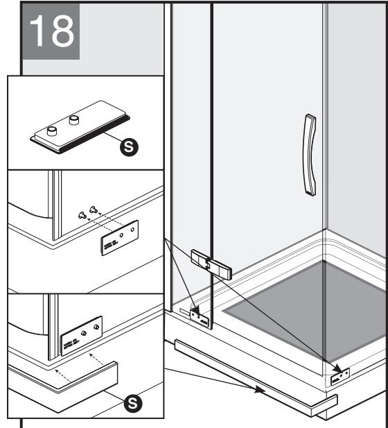
**S** Apply a bead of caulk to the bottom of the plastic spacer. Install plastic spacers onto glass panels.
