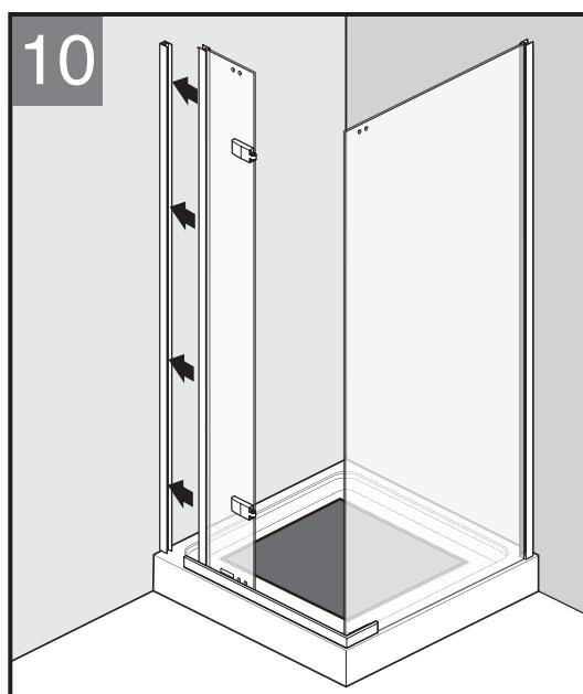
Insert the small glass panel over the wall jamb.
