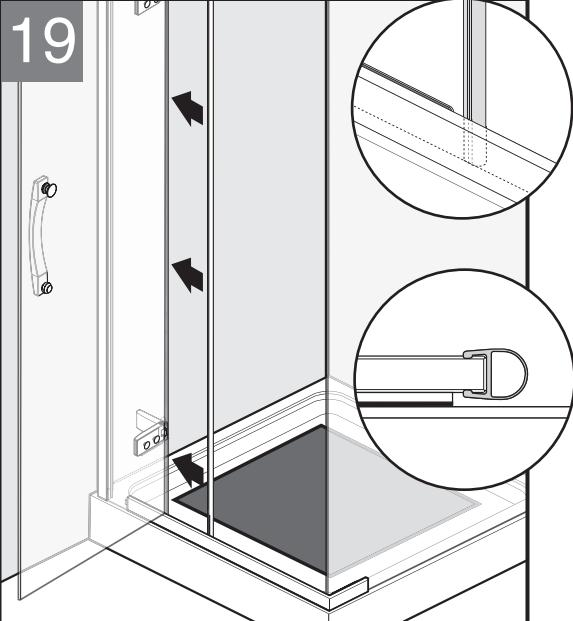
Starting at the bottom, press the bulb gasket onto the edge of the small glass panel.
