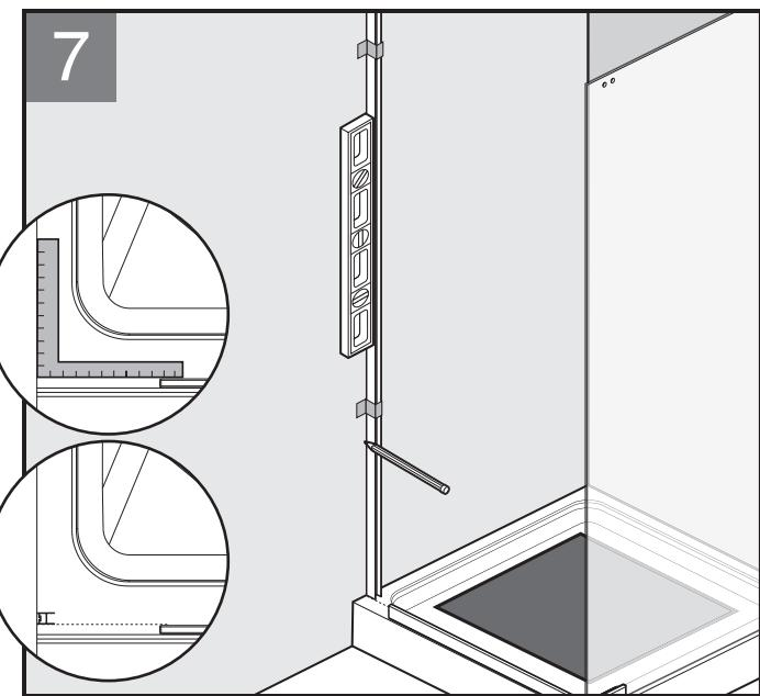
Place a framing square on the base, lined up with the support bar and opposite wall. Make sure that the support bar is even with the front edge of the base, and mark a line on the wall. Position the wall jamb so that the outer edge is even with the marked line. Hold it in place with tape. Check that the wall jamb is plumb.
