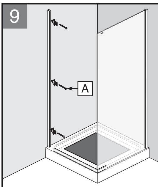
Install wall jamb using (3) M4 x 38mm screws [A].
