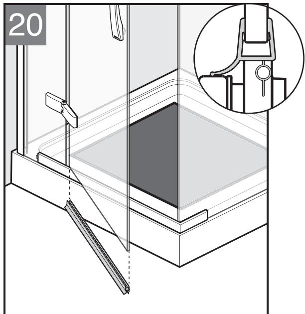
Starting on one end, press the sweep gasket onto the bottom of the door. Make sure the ends of the gasket are flush with the glass.
