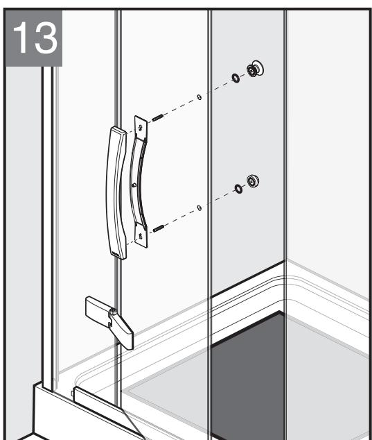
Install handle. Make sure that O-rings are in place on the inside of the door.
