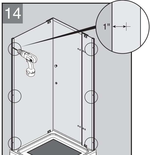
From inside the shower, drill three pilot holes into each glass panel frame and wall jamb using 1/8" drill bit. Holes should be 1" from the wall and spaced as shown.
