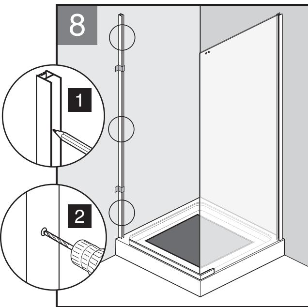
Mark (3) hole locations and remove wall jambs. Drill holes through wall material using a 3/16" drill bit (for tile walls, use a glass and tile bit). Then use a 9/64" drill bit to drill holes into studs.
