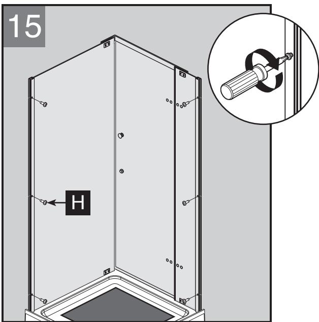
Secure the glass panel frames to the wall jambs using (6) M4 screws [H].
