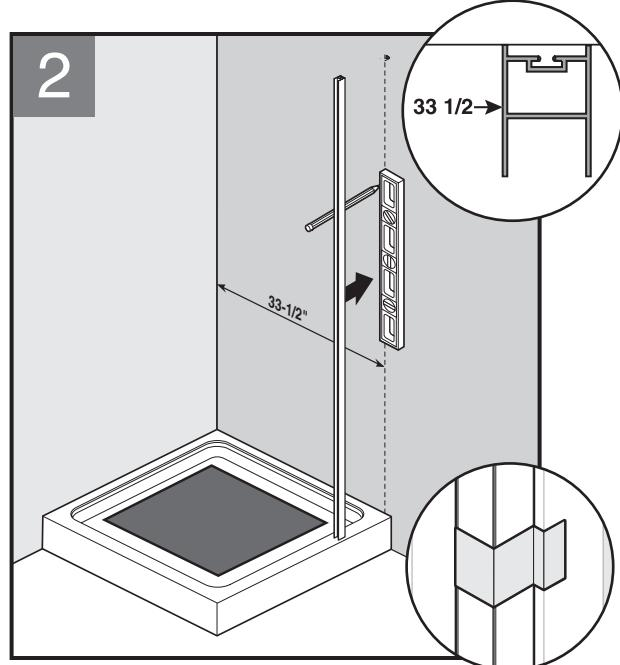
The wall jamb for the large glass panel will be installed first. Measure 33-1/2" from the opposite finished wall and mark a line. Using a long level, extend a plumb line up the wall.
