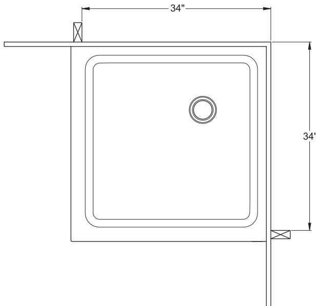
Studs must be in this location on each side for door installation.
