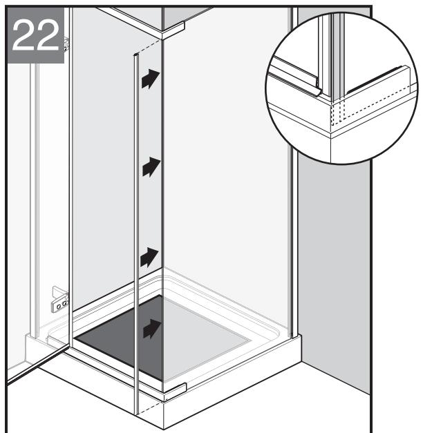
Starting at the bottom, press the magnetic gasket onto the edge of the large glass panel.
