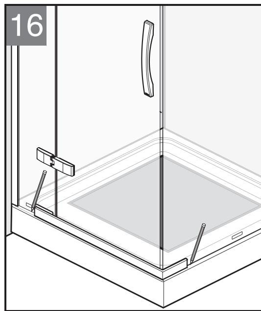
Mark a pencil line or use tape to mark the location of the glass panels on the base.
