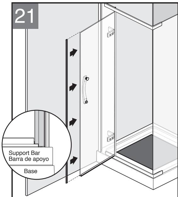
Starting at the bottom, press the magnetic gasket onto the edge of the door. Make sure there is little to no gap between the bottom of the gasket and support bar, and that the gasket doesn't rub on the bar.
