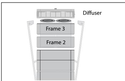
1. Open the locking arms, remove the diffuser and frame 3.
