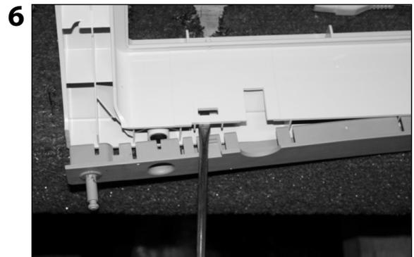
Use the screwdriver to gently loosen and lift the rail away from the base. Lift the rail out by hand. Repeat steps 5 and 6 for the second rail.
