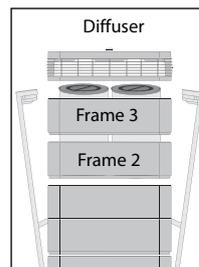
6. Replace frame 2 with the cartridges, the other frame, and the diffuser. Close the device by pressing both arms together. Reset filter life (refer to section 4.4.8).
