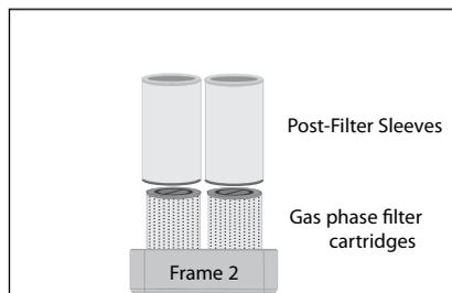
2. Frame 2 contains the four gas phase filter cartridges with the four Post-Filter Sleeves. Remove frame 2 with the cartridges.
