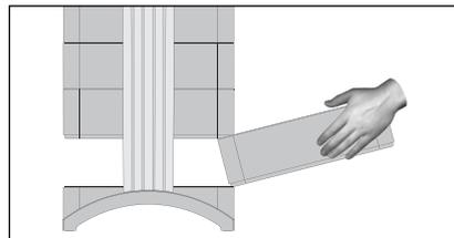
11. To reinsert frame 1, tilt it upwards at an angle while progressively pushing the frame back into the housing. For details on how to close the housing, please refer to section 6.3.
