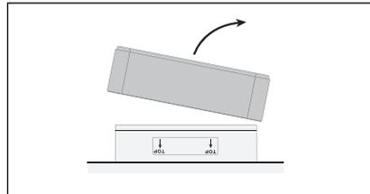
8. Dispose of the used filter by placing it into the plastic bag in which the new filter is supplied (see section 6.6).
