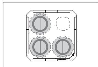
3. To remove the cartridges, twist each cartridge counter clockwise as far as it will go. It can then be lifted out of the base plate by hand (disposal see 6.6).
