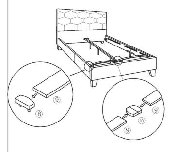
Connect one of each slat, part (9), with one, part (8), Then connect, part (9), to part (10)
