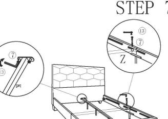
Use Allen Key, part (13), to secure bolts, parts (7) 4pcs, to connect, part (K), to parts HB&FB.
