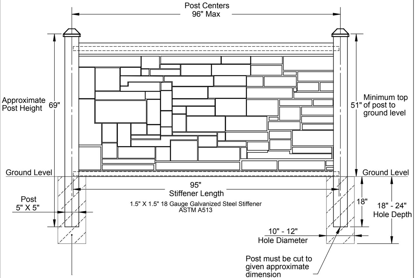
Concrete footing diameter 10" to 12" min and 18" to 24" deep min in accordance with local conditions, codes, and standard building practices.
