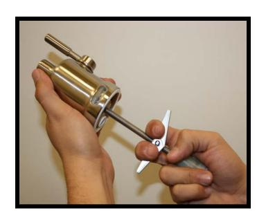
During shipping the toggle bolt on your new faucet may push up out of position. Prior to installing hold the faucet as shown in the picture pull down on the wing nut this will make sure the orings are in their proper position and your faucet will have a good seal.
