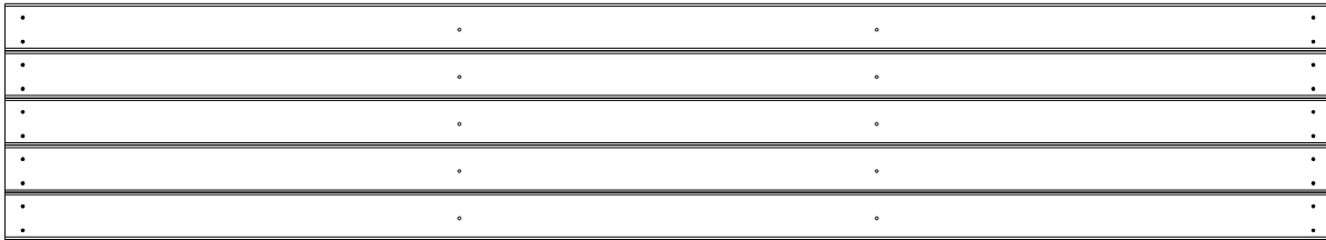
(1) RP2 - ROOF PANEL - W2A02513 1 9/16"x15 3/4"x86 7/8" (40x400x2206)
