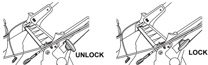
2. Turn the adjust knobs 90 degrees into the lock position so the pins will spring into the holes and lock into position.
