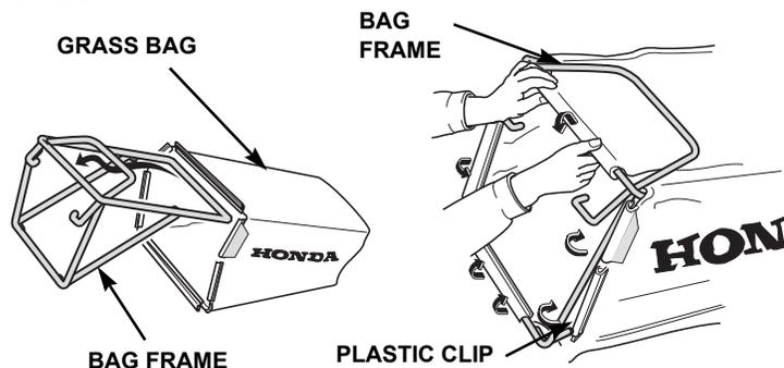
Lift the discharge guard, remove the mulching plug, and install the grass bag.
