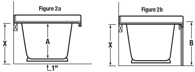
For installations that are any combination of decks, walls, and pony walls, use the same methods to determine critical heights. Remember that all supports must be at the same height and must establish a plane that is level front to back and side to side.
