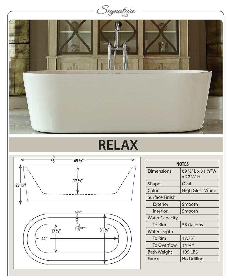
Actual dimensions may vary + /- 1/2" due to variations in the manufacturing process. Measurements for rough-in must be taken directly from the bath.
