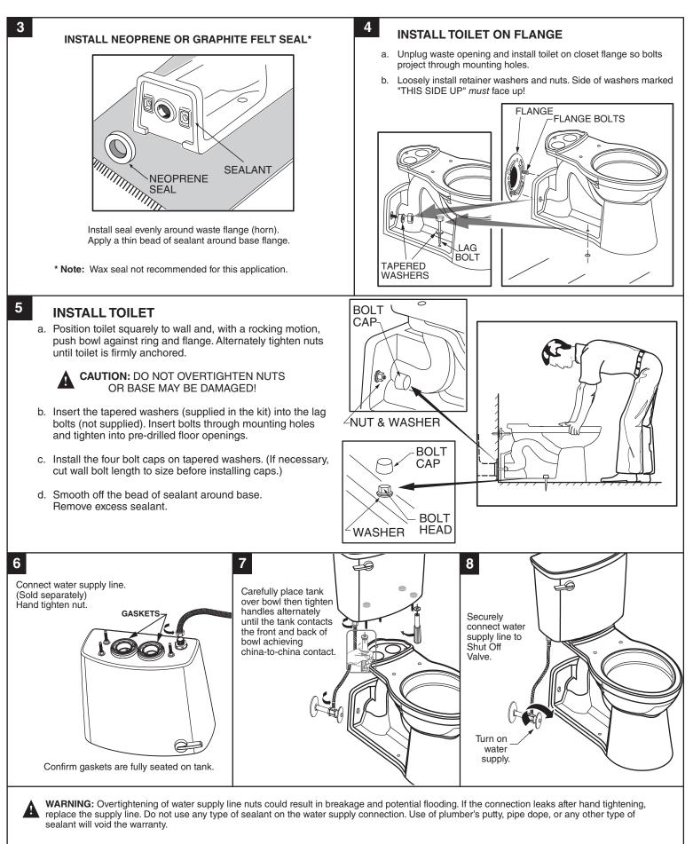
WARNING: Do not use plumber's putty, pipe dope, or any other sealant on the water supply connection to this tank. If the connection leaks after hand tightening, replace the supply line. If the connection continues to leak with the new supply line, replace the fill valve. Warranty is void if any type of sealant is used on the water supply connection.
