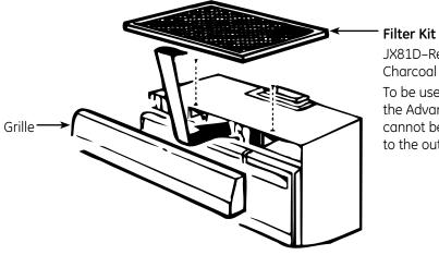
JX81D-Recirculating Charcoal Filter Kit To be used when the Advantium oven cannot be vented to the outside.
