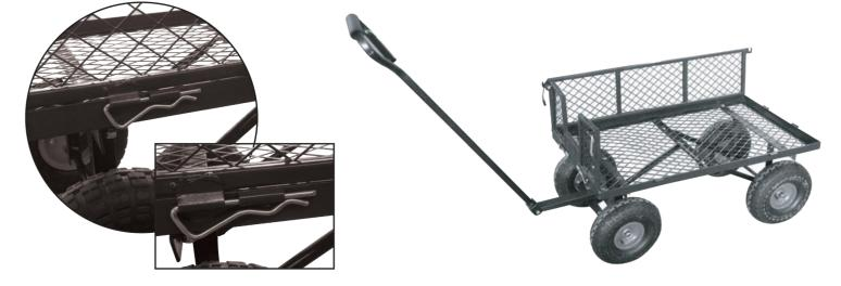
8. To lock the Sides in place, hold Side Panel in the up position. Rotate Side Panel Lock Lever from the up position to the down position and in doing so capture the Side Panel hook.
