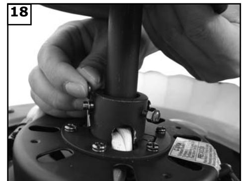
18 Align hole in downrod with hole in yoke and install cross pin. Install downrod assembly into yoke. Install keeper into cross pin.
