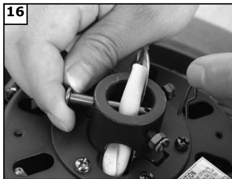
16 Remove keeper from cross pin and then cross pin from yoke. Replace keeper on cross pin and save.
