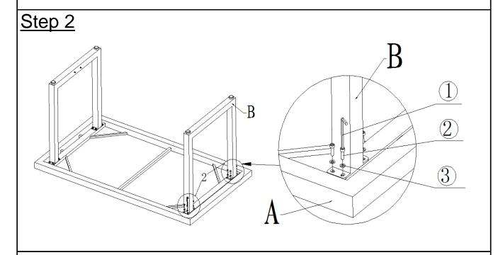
Attach the other Table Leg(B) to Table Top(A) using Bolts(2) and Washers(3) with Allen Key(1).
