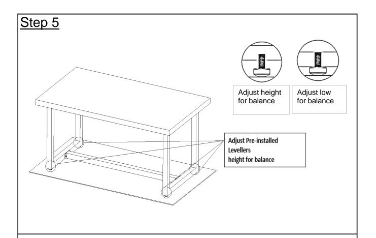
Place the Table on a level surface. Adjust the Legs pre-installed Levellers until the Table is level with the ground.
