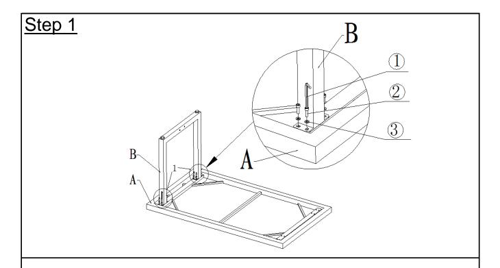
Position the Table Top(A) facedown on a clean, non-marring surface. Attach Table Leg(B) to Table Top(A) using Bolts(2) and Washers(3) with Allen Key(1).
