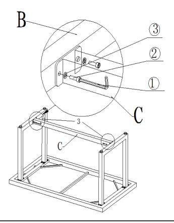
Insert the Leg Connector(C) between the Table Legs(B).
