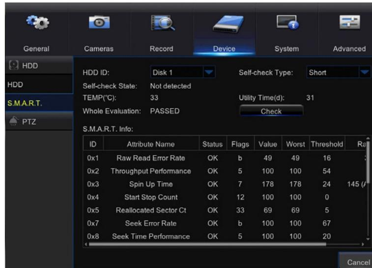
**HDD ID:** Allows to select the Hard Drive that is going to be checked or just select the Hard Drive to see it's statistics.
