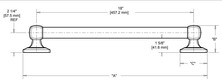
MATERIALS: Grab bar is constructed using 1-1/4" diameter 20 gauge 304 stainless steel tubing.
