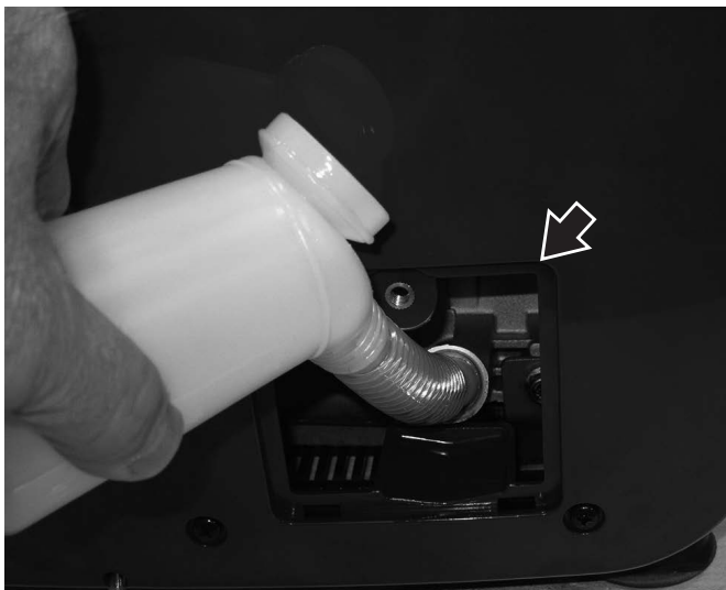
Figure 24 – Adding Engine Oil
