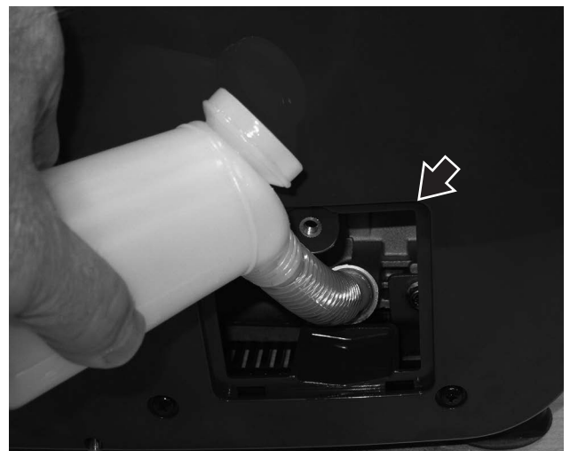
Figure 38 – Adding Engine Oil
