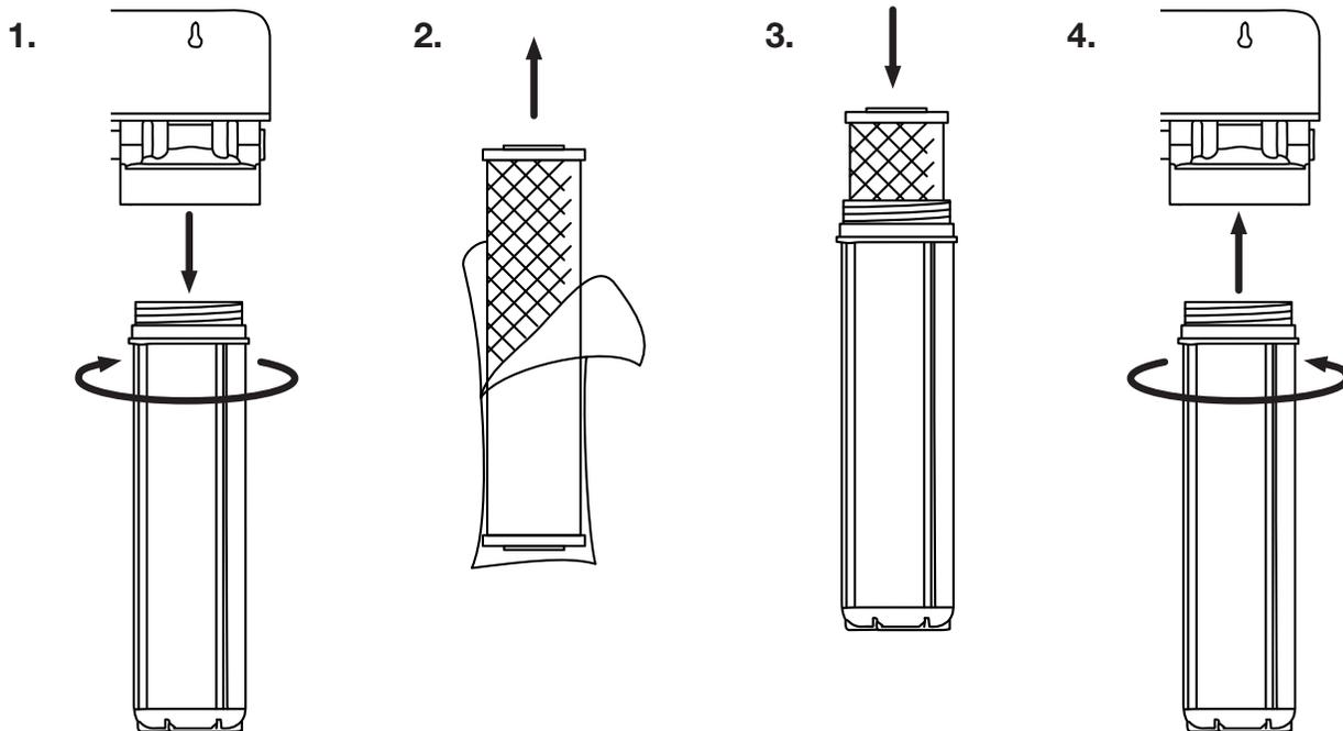
**Remove both filters from sumps,
