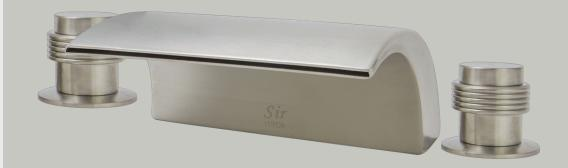
7" x 5 1/4" x 2 7/8" 3-Hole Installation 6" - 24" Centerset 1/4-Turn Washerless Ceramic Cartridge Completely Pressure Tested ADA Approved Lifetime Warranty PVD Brushed-Nickel Finish
