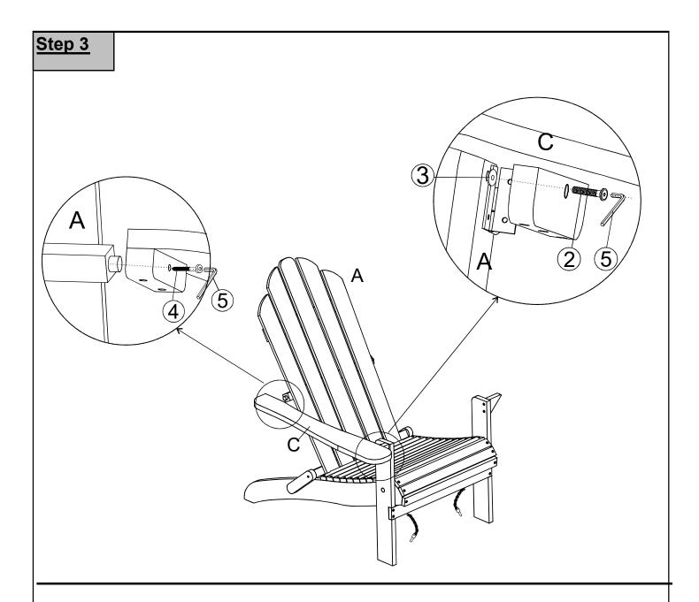
Insert Left Armrest(C) onto tenon on Backrest Support and attach using Screw((4)) with Allen Key((5)).
