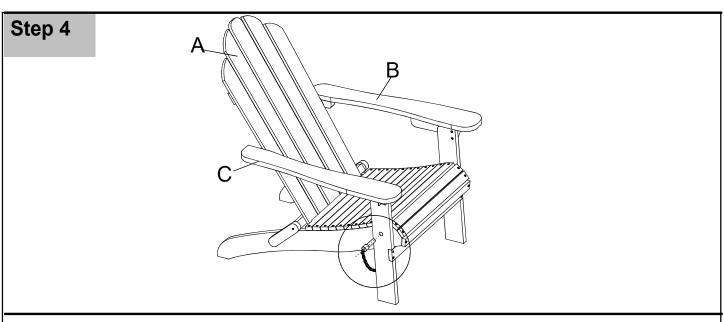
Push the Wooden Pin through the Legs as pictured to Lock the Chair into position. Gently and gracefully, sit onto to the Adirondack Chair. This will help to align all the parts at all joint areas.
