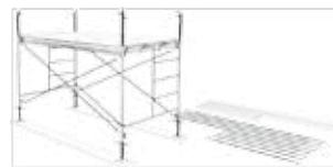
Install the guardrail posts onto the coupling pins seated in the top of the frames. Put a pig tail lock through the top and bottom of each coupling pin to avoid any separation.
