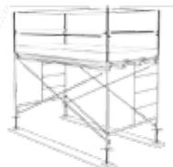
Install toeboards as required. The gap between the bottom of the toeboard and the top of the platform must not be more than 1/2 inches.
