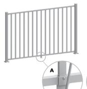
Fasten the second post to the concrete surface (see Step 1). Install bottom rail support:
