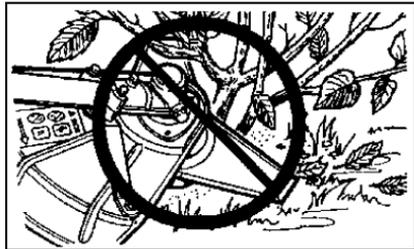
**8 Tooth Weed/Grass Blade** is designed for grass, garden debris and thick weeds up to 19 mm (0.75 in.) diameter. DO NOT use this blade for brush or heavy woody growth.
