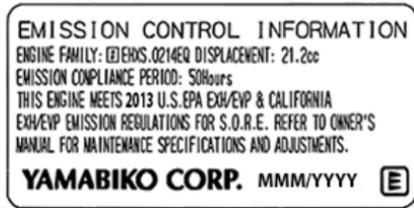
An Emission Control Label is located on the engine. (This is an EXAMPLE ONLY, information on label varies by engine FAMILY).
