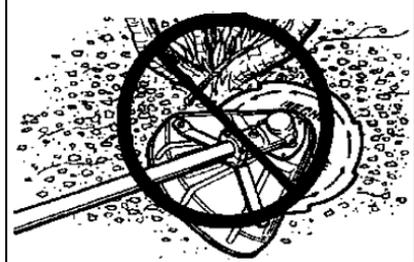
**80 Tooth Brush Blade** is designed for cutting brush and woody growth up to 13 mm (0.5 in.) diameter.
