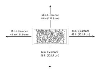
Combustible materials should not be within 72 inches of the top of the unit, or within 48 inches around the entire unit.
