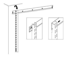
Assemble with hang rail slotted ends to outside. Make sure notches are at the far end of assembled hang rail and space the hang rails on the Top Track 30-3/8" apart measured inside (between) the hang rails.
