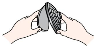
Pull the top piece of the Dome Filter off and remove the foam media. Shake it out, rinse it, and let it air dry thoroughly.
