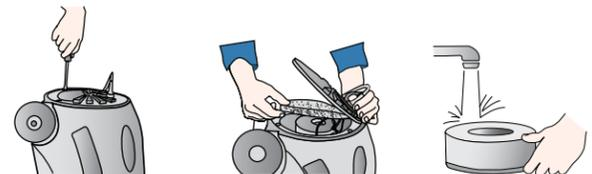
Once a month (or more often if necessary) clean the exhaust diffuser. With a Phillips screwdriver, remove the four screws from the vented exhaust cover. Pull back the cover and remove the foam diffuser. Rinse the diffuser, and let it air dry thoroughly. Before the next use, return the diffuser to its place.
