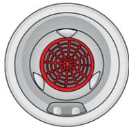
Once a week, or as necessary, clean or replace the Dome Filter. First, remove the Intercept Micro Filter and Cloth Filter. Reach into the vacuum body and twist dome filter from motor.
