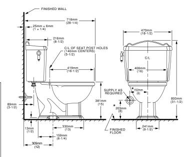
THIS COMBINATION IS DESIGNED TO ROUGH-IN AT A MINIMUM DIMENSION OF 305MM (12") FROM FINISHED WALL TO C/L OF OUTLET.
