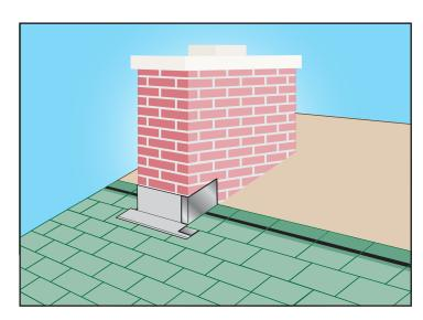
2. Install the next course of shingles, covering the corner piece installed in Step 1.
