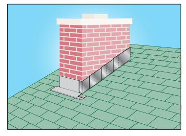
4. Continue interweaving the Step Flashing and shingles. Protect the top edge of the step flashing with caulking or metal counter flashing.
