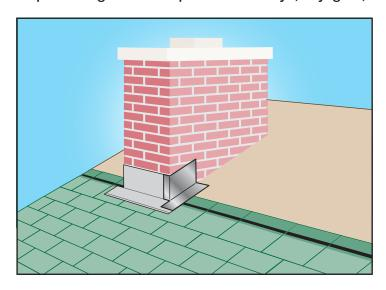
1. After shingling up to the chimney and installing the base flashing, cut and bend a piece of Step Flashing to make a corner piece. Secure with 2 roofing nails.
