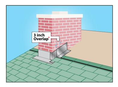
3. Position the next Step Flashing piece snug against the chimney and overlapping the previous piece by 2-3 inches. Secure with 1 roofing nail, then complete the course of shingles. \*Check local building code.
