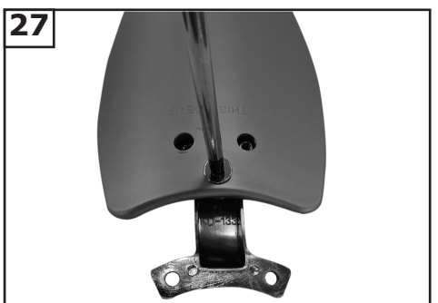
27 Place blade holders onto blades aligning holes in blade holder with holes in blade. Make sure that the side of the blade you select is facing downward. Install 3 screws to back side of blade as shown. Tighten screws securely. Repeat this process 3 more times until all blades are assembled.
