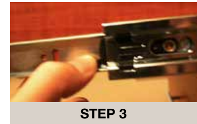
For slide on right side of drawer box locate the black tab and push DOWN to release. With both tabs released at same time slide out the drawer.
