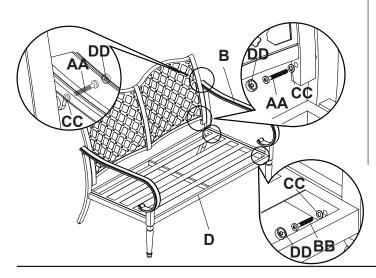
□ Attach the loveseat back (A) to the right arm (C) using M6 bolts (AA) and washers (CC).
