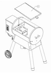
**POSITIONING THE PORCELAIN GRILL** Insert Porcelain Grill (135) into Grill Frame Body (1) and rest on angles centered front to back and side to side.
