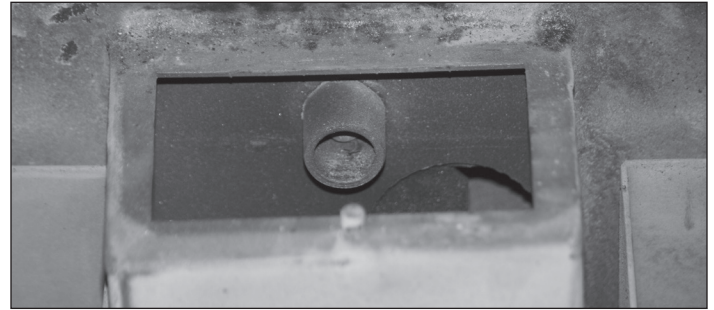
Figure 34: Remove ash from ignitor tube (underneath firepot)
