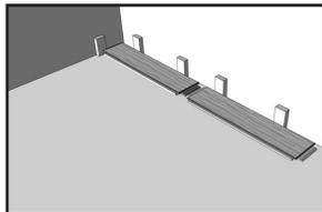
**STEP 2 –** Use a laminate flooring tapping block to gently tap second plank against the short side to join plank A and plank B.
