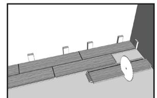
**STEP 2 –** Flip the plank back over (décor side up) so the tongue faces the groove of the adjacent plank; install as shown in step 4.
