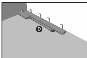
**STEP 5 –** Once plank is flat, gently tap the second plank against the short side of plank C, joining plank C and D.
