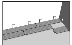
**STEP 3 –** Tap the two sides together using a pull bar. If the remainder of the previous plank is at least 12 inches long, use it to start the next row.
