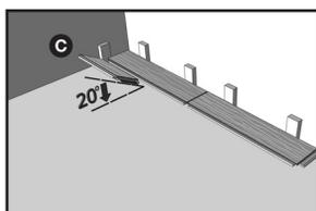
**STEP 4 –** The next plank (plank D) should be installed with the tongue on the left side of the plank next to the previous plank. Push plank flat to the floor as in step 3.
