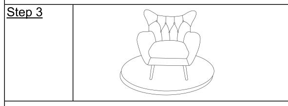
Place the chair on a LEVEL SURFACE to see if it wobbles. If it wobbles, press firmly down on both armrests at the same time. This will help to ensure all Bolts and gaps reach full alignment status.
