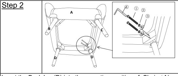
Insert the Back Leg(D) into the mounting position of Chair (A). Attach the Back Leg(D) using Bolts(1), Spring Washers(2) and Washers(3)with Allen Key(4).
