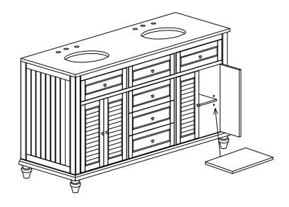
To adjust the shelf, please use a screwdriver to remove the 4 screw inserts and shelf support brackets which are under the shelf. Move the shelf and place the support bracket into the pre-drilled insert holes. Then secure with screw inserts.
