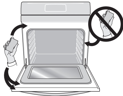
Figure 17: Clean around the oven door gasket
