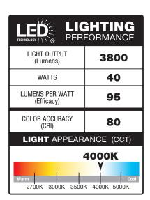
All results according to IESNA - LM79-2008 Light Output reported as total integrated lumens (light source & fixture)
