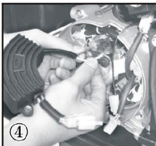
④ Take down the AVR from carbon-brush
